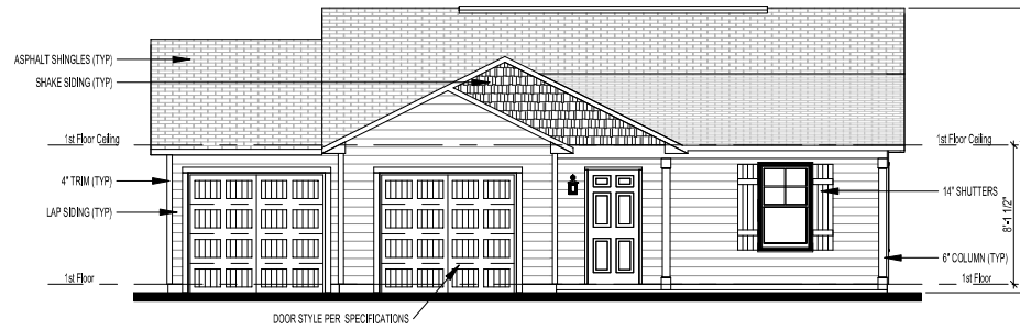
① Front Elevation - Elev B - 2 Car Garage 1/8" = 1'-0"
