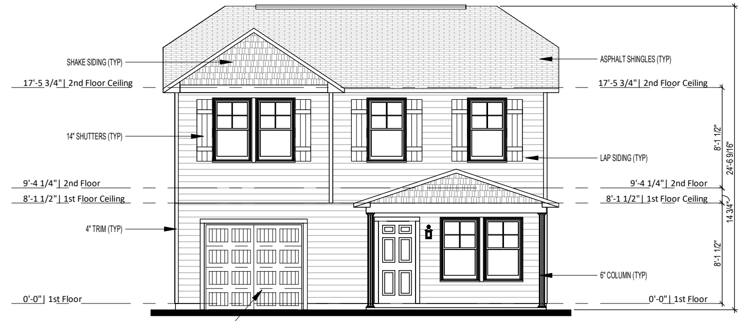
① Front Elevation - Elev B - 1 Car Garage 1/8" = 1'-0"
