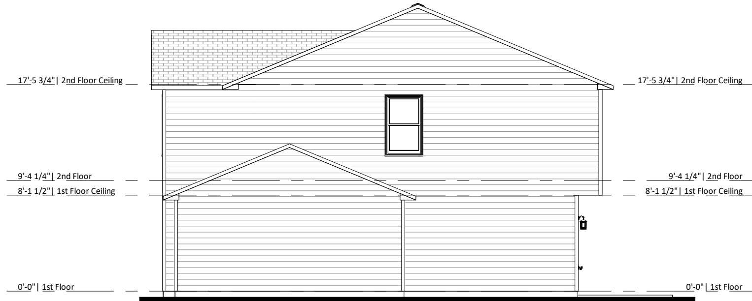
① Right Elevation - Elev A - 2 Car Garage 1/8" = 1'-0"
