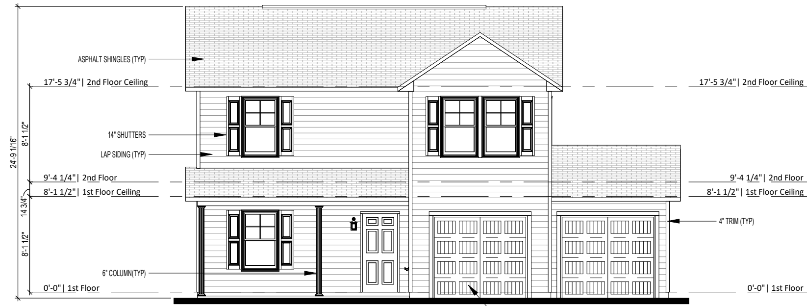
① Front Elevation - Elev A - 2 Car Garage 1/8" = 1'-0"
