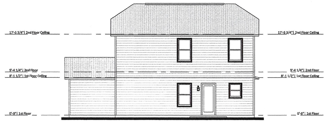
② Rear Elevation - Elev B - 2 Car Garage 1/8" = 1'-0"
