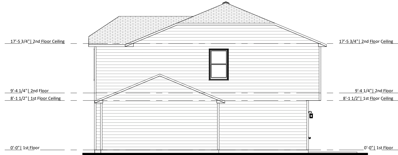
① Right Elevation - Elev B - 2 Car Garage 1/8" = 1'-0"
