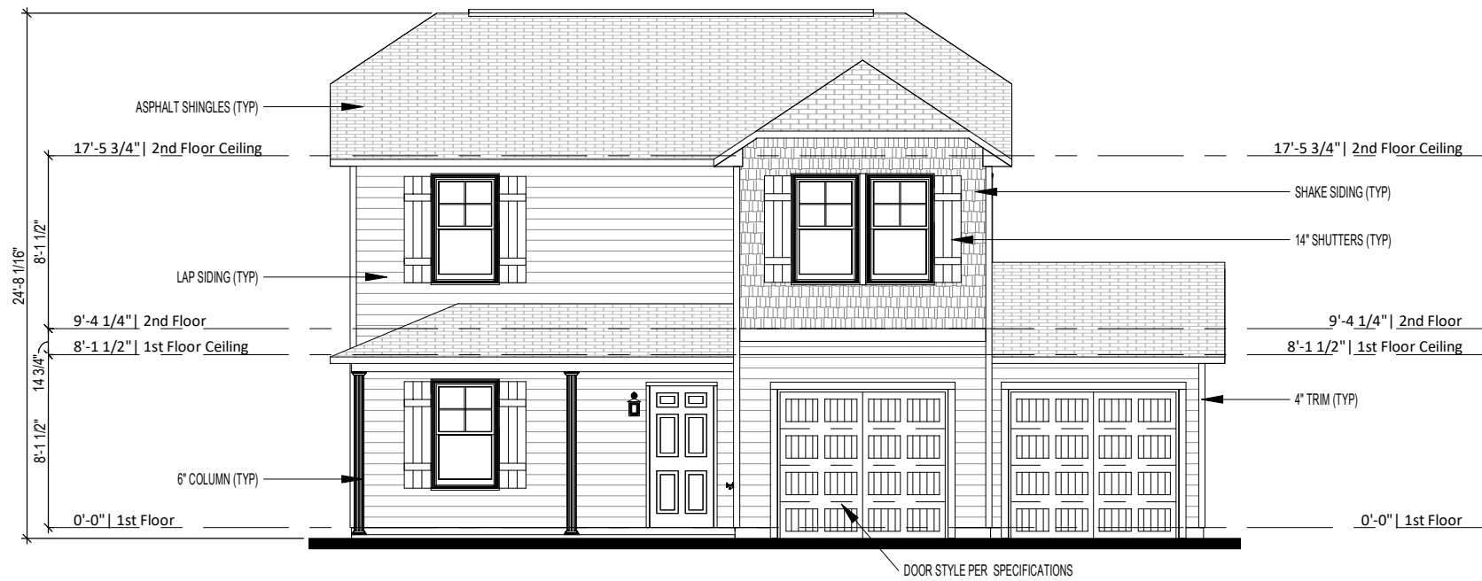
① Front Elevation - Elev B - 2 Car Garage 1/8" = 1'-0"
