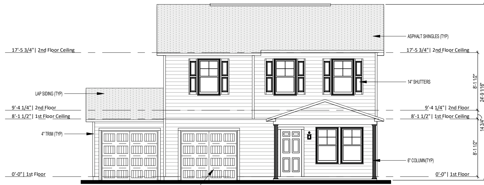
1 Front Elevation - Elev A - 2 Car Garage 1/8" = 1'-0"
