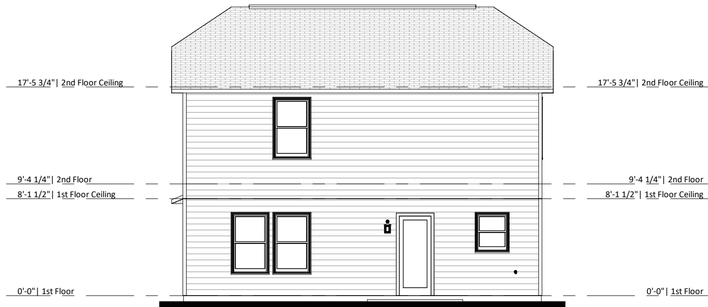
2 Rear Elevation - Elev B - 1 Car Garage 1/8" = 1'-0"
