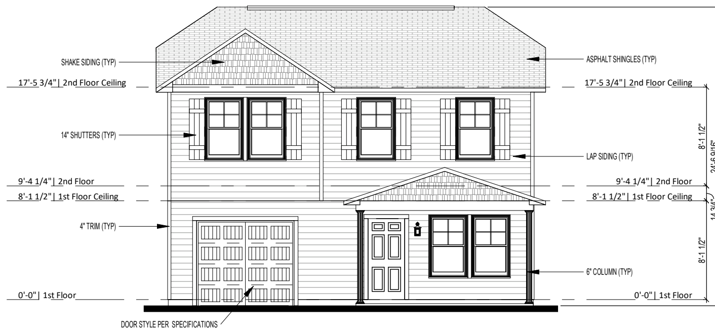
1 Front Elevation - Elev B - 1 Car Garage 1/8" = 1'-0"
