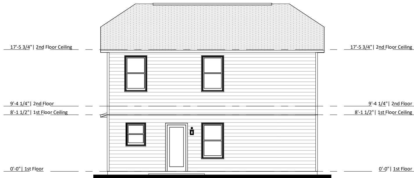
2 Rear Elevation - Elev B - 1 Car Garage 1/8" = 1'-0"
