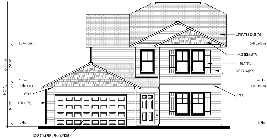
① Front Elevation - Elev B 1/8" = 1'-0"
