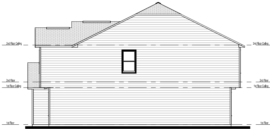
① Right Elevation - Elev B 1/8" = 1'-0"
