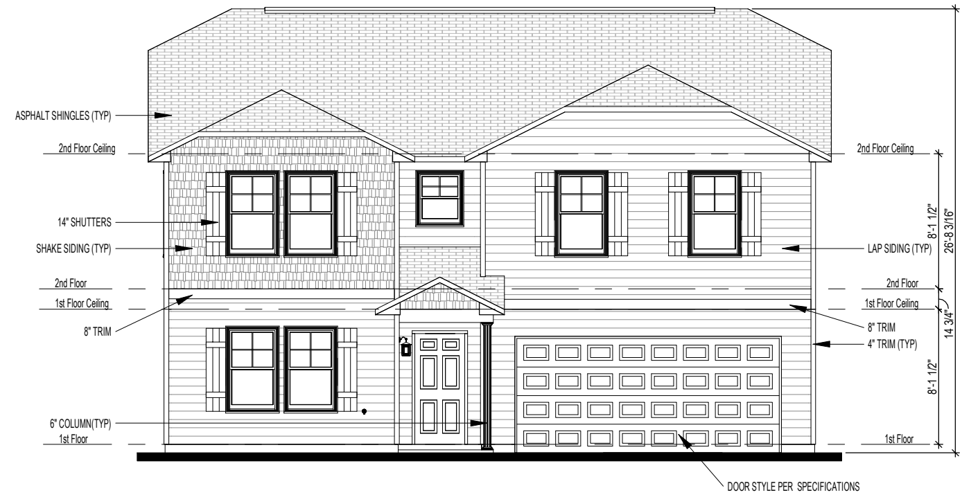
① Front Elevation - Elev B 1/8" = 1'-0"
