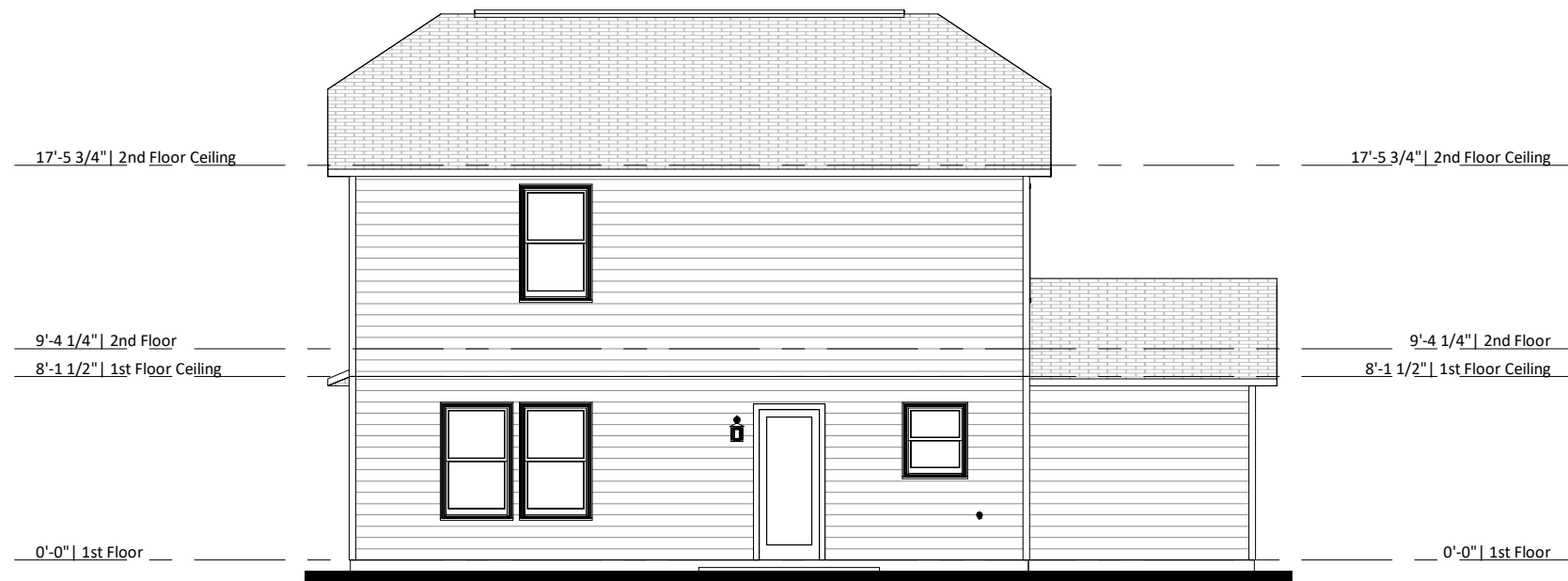
2 Rear Elevation - Elev B - 2 Car Garage 1/8" = 1'-0"
