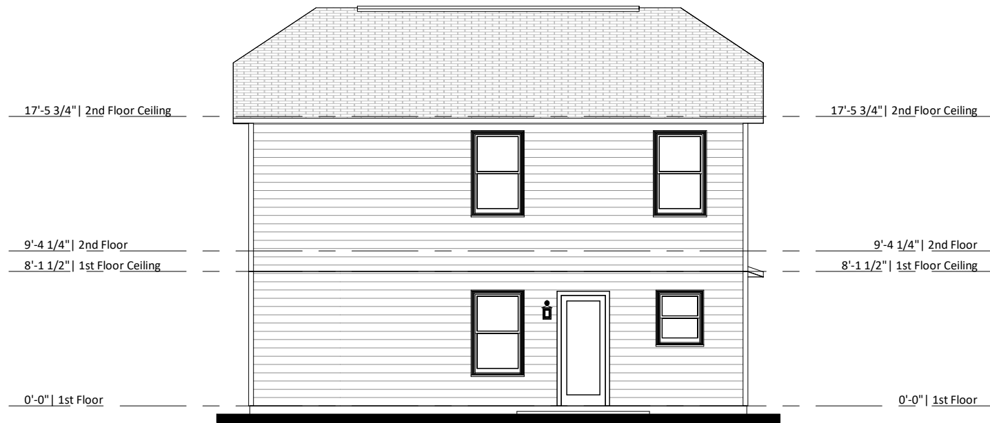
② Rear Elevation - Elev B - 1 Car Garage 1/8" = 1'-0"
