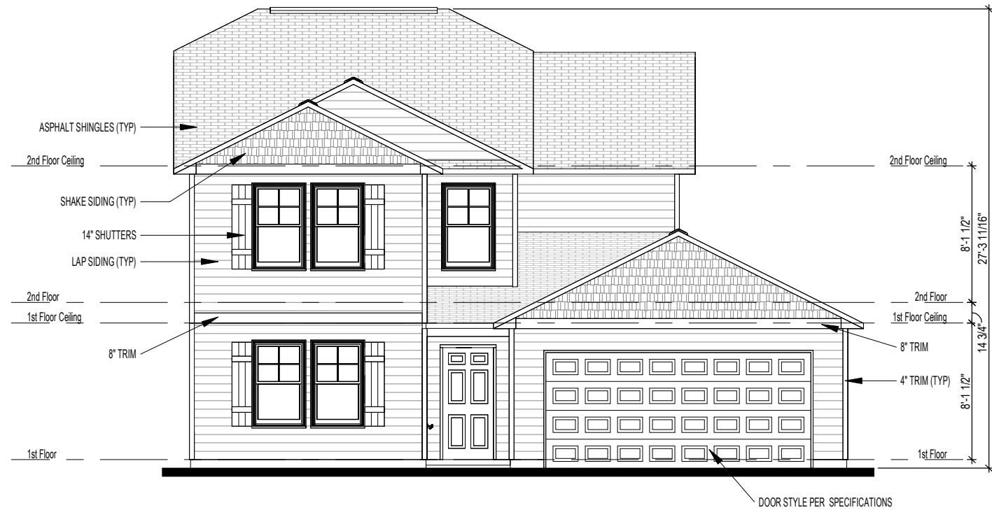
1 Front Elevation - Elev B 1/8" = 1'-0"
